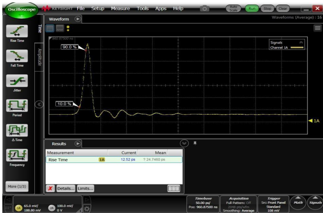
Figure 3-2 HSPD4018 Pulse Response Curve
