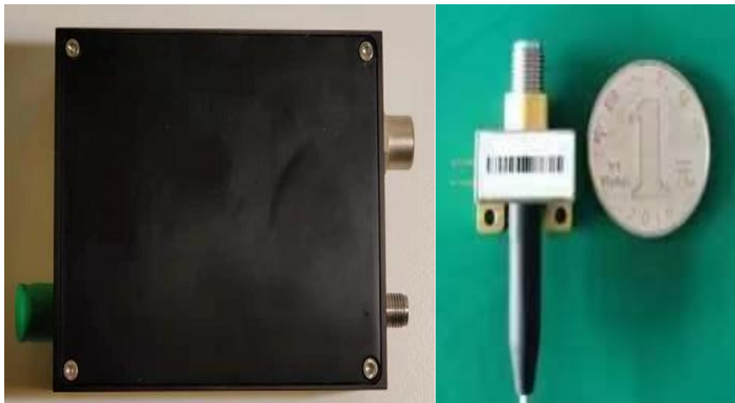
Figure 2-1 Detector Module Appearance (Left), High-Speed Bare PD (Right)
