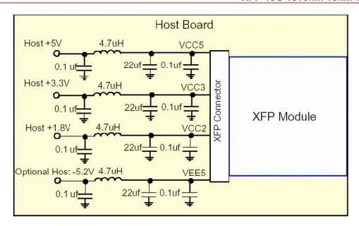
Recommended Host Board Power Supply Circuit
