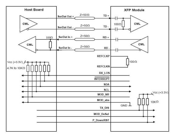
**Recommended High-speed Interface Circuit**
