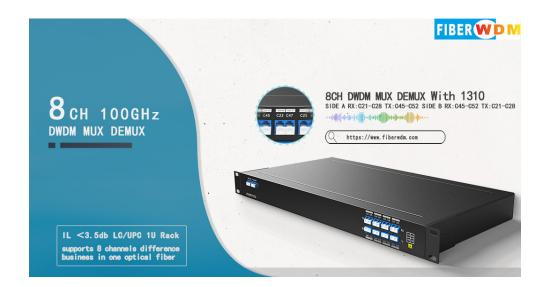
The 8ch(16waves) DWDM MUX/ DEMUX with 1310nm is used in pairs, designed by FIBERWDM, in side A, the waves are: RX C21 to C28(1560.61nm~1554.94nm), TX C45 to C52(1541.35nm~1535.82nm); And in side B, the waves are: RX C45 to C52(1541.35nm~1535.82nm), TX C21 to C28(1560.61nm~1554.94nm).
